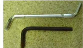
Allen wrench. So if you cannot find yours, use the appropriate size Allen wrench. Stick the short end into the matching hole in the bottom center of the disposal and use the long end to turn it back and forth until you break free whatever's got the disposal stuck.
